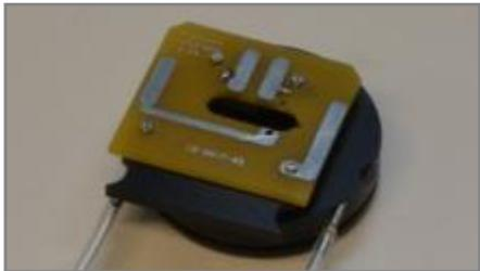
Cell closed, sealed and ready to insert into the TT-AFM light lever.
